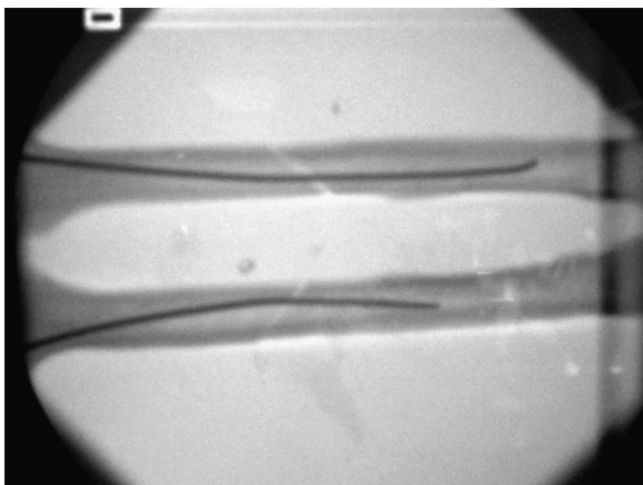
FIGURE 2. Radiographs of canine radii comparing 3- and 5-diameter insertion lengths and illustrating the 3-point bending fixation technique.
